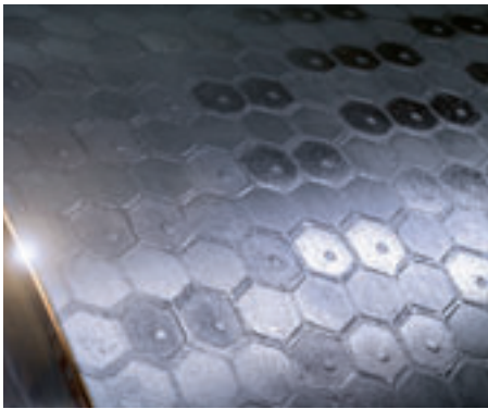
HEXADUR® standard surface and electrochemically machined, preconditioned surface
