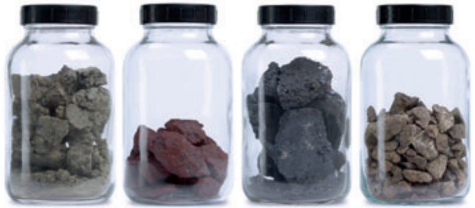
Test work materials for grinding: cement clinker, iron ore, blue lead, diamond ore
