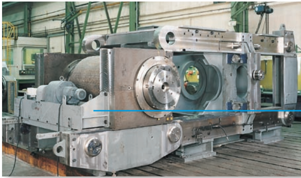
Roller pulling with roller removal device
