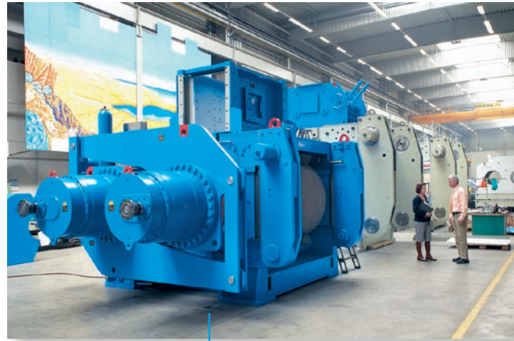
Final assembly of roller presses in Köppern's workshop
