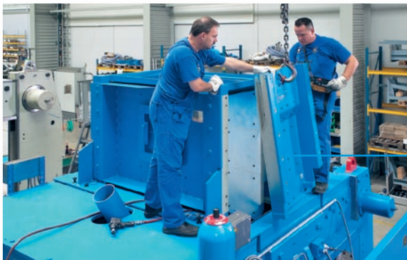
Feed box with exchangeable wear lining
