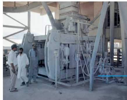
HPGR for limestone-grinding, Pakistan
